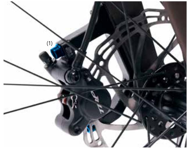
Alternatively, you can also try to align your brake caliper over the disc by pulling the brake lever. The brake pistons make contact with the disc via the brake pads and align the loosely screwed-on brake caliper in the center above the brake disc. With the brake pulled, you should now tighten the screws (1) again and make sure that the caliper does not move again.
