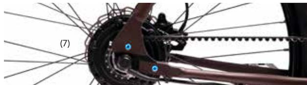
The rear wheel will move closer to the left chain stay if you screw the belt tensioner bolt in further on the left side, or loosen it a bit on the right side, and vice versa. When the rear wheel is centered again, you have to tighten the four screws of the slider plates again with the appropriate torque (see *chapter Tightening Torques*).
